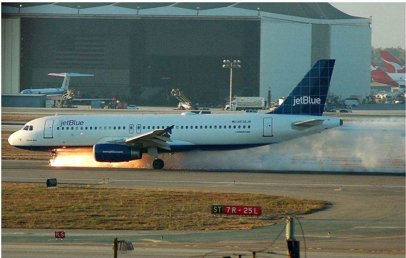
Wikipedia / Image by Andrew Marino / JetBlue Flight 292 - 21 Sep 2005. The 8 crewmembers and 140 passengers of this Airbus A-320 were not injured during this spectacular landing (nose-wheel stuck down at 90 degrees to aircraft's fore and aft axis)
